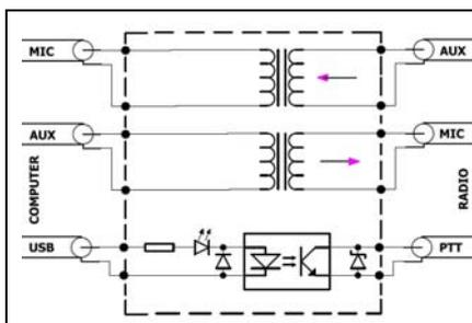
Input and output audio signals from the radio to the computer and vice versa are supplied through 1:1 bidirectional audio transformers for proper isolation of the circuit.
